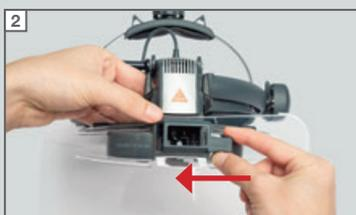
Take the mounting clip supplied and push it onto the guide tab on the instrument.
