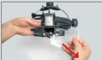
For cleaning and disinfection, remove both the transparent Breath Shield and the mounting clip from the instrument.
